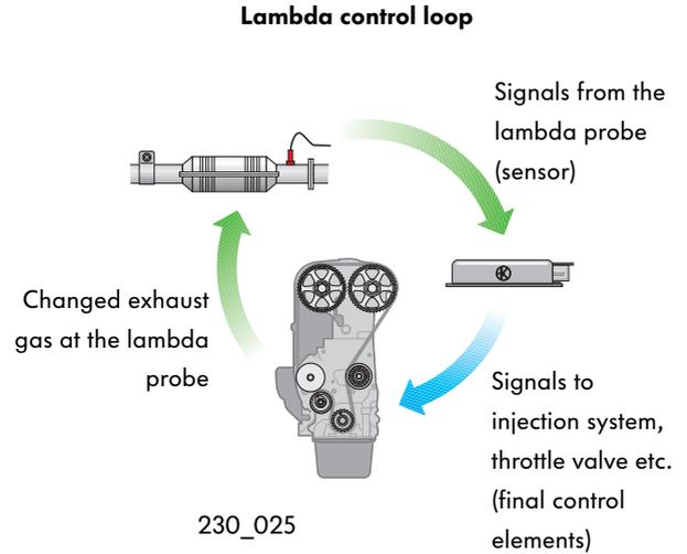
The catalytic converter is able to clean the exhaust gases at a temperature of approximately  $300^{\circ}\text{C}$  or higher and needs a certain amount of time to heat up after a cold start. To shorten the warm-up phase and clean exhaust gases more quickly, primary catalytic converters are used in modern exhaust systems. They are located near to the exhaust manifold. They are normally small in size, and so reach their operating temperature more quickly.
