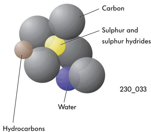
The particulate matter typically emitted by a diesel engine comprises a core and several attached components, of which only the hydrocarbons (HC) are oxidised in the oxidation catalytic converter. The residues of the particulate matter can only be collected by special particulate filters.
